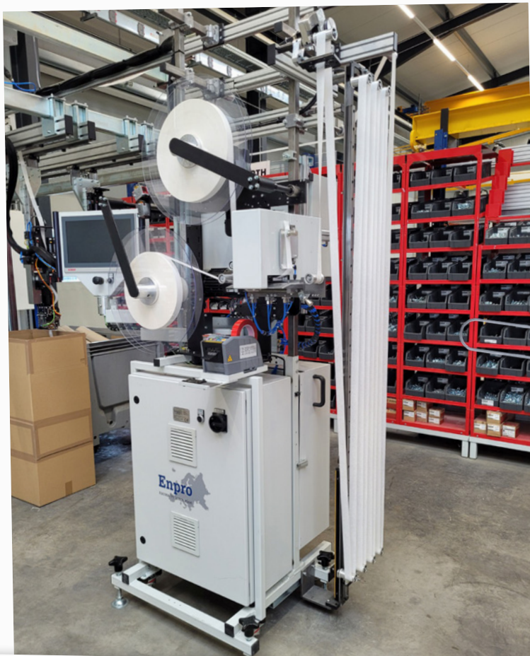
Enpro Splicer: changing disk rolls at full production speed
